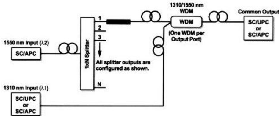
**Narrowcast Module High Isolation, Rack Mount,
