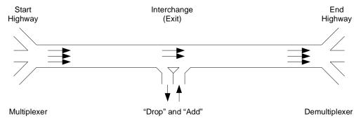
The Mux module serves the same purpose as the beginning of the highway. Multiple roads combine into the one controlled highway. Each road is like a different wavelength, or channel. The Mux module combines, or *multiplexes*, multiple wavelengths onto a single fiber.
