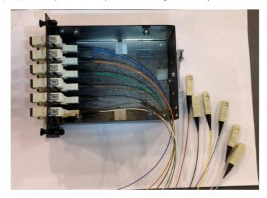
4. Once the panels are populated, manage the fibers into the rings and secure cable jacket with two zip ties. Photo is shown without black shrink for clarity of zip tie positioning. Do not zip tie onto the 900um fibers. Replace cover and screws.
