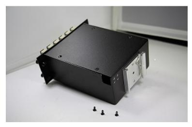
2. Remove lid and observe notch (lower right in this photo) for cable entry. Orient the Multimount LGX patch panel module so that the fiber cable enters without twisting or kinking and so that the DIN clip is positioned toward the DIN rail.
