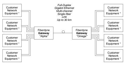
\* Note: Customer Equipment can be any mix of 1000Base-T, 1000Base-SX (850 nm) or 1000Base-LX (1310 nm)
