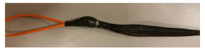
At the other end, where the mesh is taped to the cable jacket, you will see a short white string. Grasp this string with needle nose pliers and use it like a rip cord to open the tape. It can be helpful to wrap the string around the pliers.
