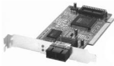
Multimode, SC, 2km, 100Base-FX, Fast Ethernet PCI Adapter Model: VS 5000
