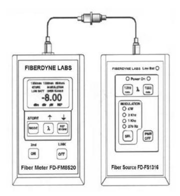
Figure 2 – Optical Power Verification Diagram
