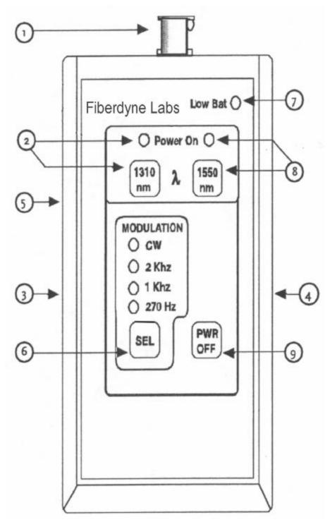
Figure 1 - FD-FS 1316 Fiber Source Front Panel
