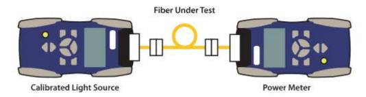
A Power Meter and Light Source combination (Loss Test Set) is the most accurate way to provide end to
