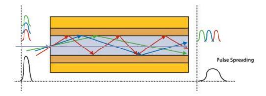
Typical CD set up would measure from 1520 nm to 1630 nm in 10 nm increments. The results are then plotted and graphed. The results include the dispersion slope, zero dispersion point and delay in ps/nm.
